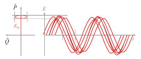
Figure 3.5.: Amplitude squeezed field
